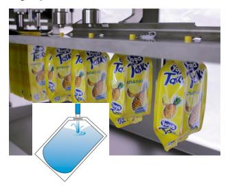
The SPOUTPRO IFC – 2 is our model for spout inserting, pouch filling through spout and capping.
